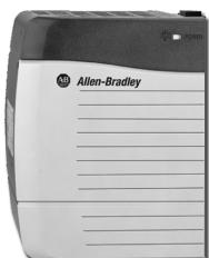
ControlLogix power supplies are used with the 1756 chassis to provide 1.2V, 3.3V, 5V, and 24V DC power directly to the chassis backplane. Select from these configurations:
